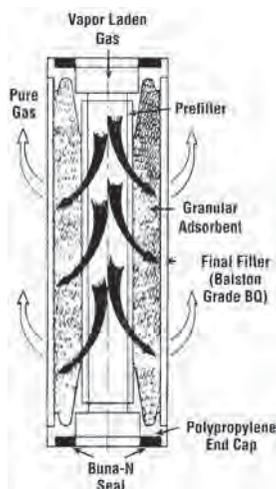
Type CI Vapor Adsorption Cartridges contain a bed of adsorbent granules in the annular space between two Microfibre Filter Tubes, with permanently bonded end caps. Utilizing a wide choice of adsorbents, the Type CI cartridges selectively remove vapors from air and other gases. Flow direction is inside-to-outside through the cartridge, and the outer Microfibre Filter cartridge serves as an integral final filter to prevent carryover of adsorbent particles.
