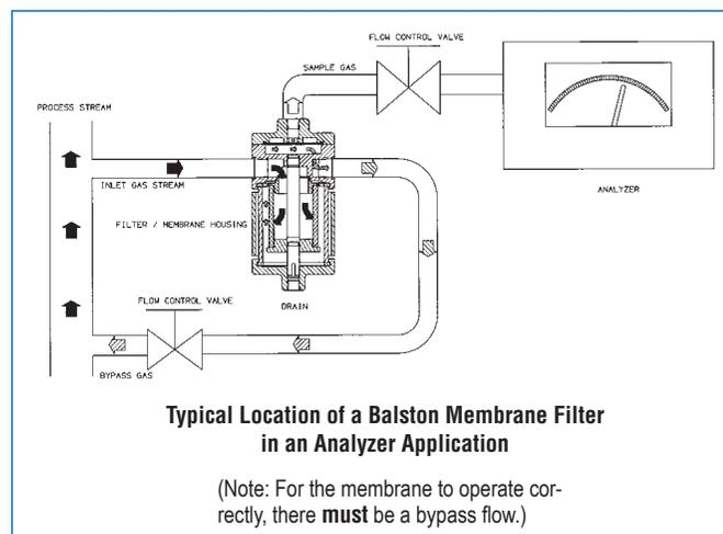
Typical Location of a Balston Membrane Filter in an Analyzer Application
